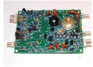
Next, I ordered a SoftRock40 transceiver kit for 40/30 meter bands. The RXTX v6.1 kit cost was \$28. I built it, and powered it up using the computer, and learned I needed a second sound card for the transceiver to work. I added a second cheap surplus 16
