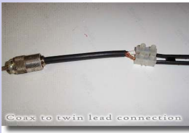
Photo E - Connection of twin lead to coax. Short length of coax section is for illustration purposes only. All connections should be weatherproofed with shrink-tubing, CoaxSeal, or similar.
