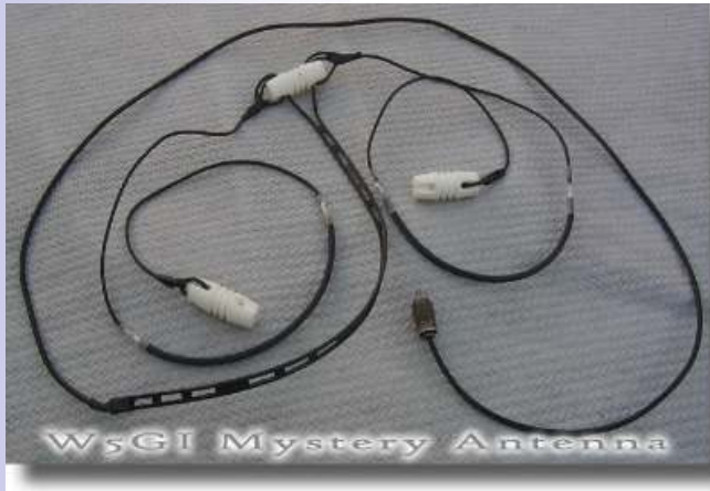
Photo A - Full view of the W5GI multi-band Mystery Antenna with all sections shortened considerably for illustration purposes.
