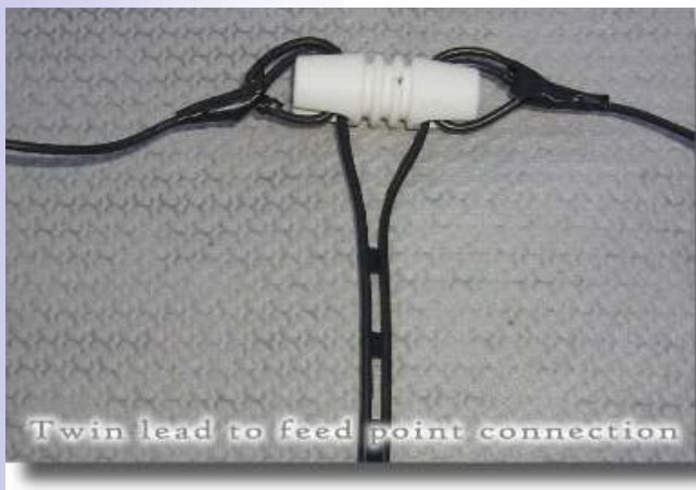
Photo D - Connection of twin lead to inner antenna wires at center of antenna.
