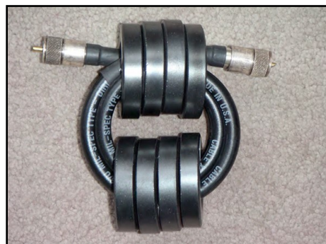
1500w common mode made with RG-213
