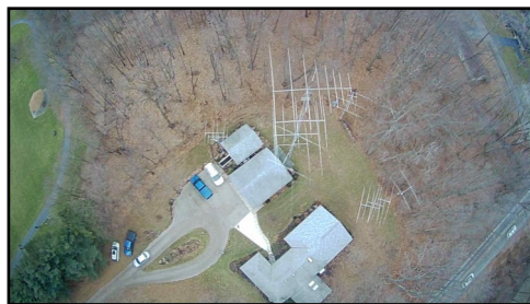
Five towers with many dipoles and yagis covering all bands 160-6m.
