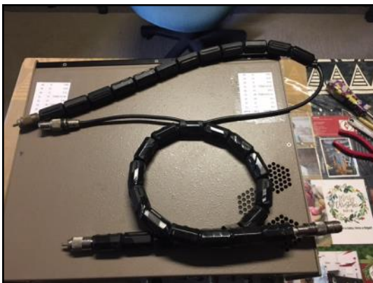
Length of coax with 12 snap-on chokes and 8 more to be added. A finished 20 snap-on choke which goes between the transceiver and amplifier.
