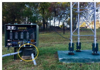
Remote switching for "each" band and the a "bypass because the tower is resonant on 75/80m
