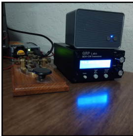
The new QRP-Labs QCX+ is on the air. Received the kit yesterday morning and, of course, built it in one session. Running 4W on 20 meters with 13.8V power supply. Made my maiden QSO today with W2LUD in WA. Lots of QSB but got a decent 559 report. The CAT interface works great with SKCC Logger. Very cool little rig. 73, Randy K5HJ
