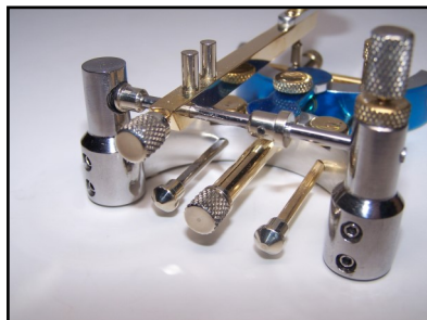
Photo #1: This shows the back end of my previously-built torsion bar straight key. The lever (rectangular rod) is attached solidly to a horizontal bar between the two upright posts (the torsion bar) which is anchored at one end and floats freely at the other. In actual use, this bar simply twists a little bit.
