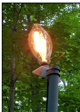
Due to SWR differences bulbs do not light the same
