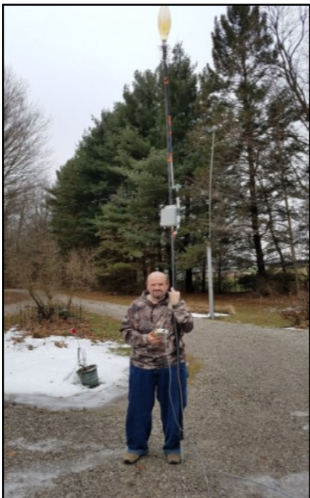
KD8VSQ with our prototype 40m antenna. The grey box is an LDG auto tuner we thought we needed but we didn’t it all and later removed it.
