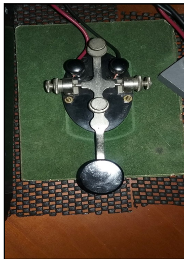
My key is an old Remler CRL 26012 WW2 vintage Navy key. I keep the gap very close and the adjustments tight. It is a pleasure to use and makes hardly any sound at all. I prefer around 20 wpm but am always ready to QRS upon request. For non-SKCC QSOs I very occasionally use the built-in keyer in my FT-450D with an old Vibrokeyer paddle, but I really don't enjoy it. For me, a well adjusted straight key is still the way to go after 52 years of experience. I'm not very likely to ever go for the TKA because I don't have a bug or sideswiper nor the funds to buy them. 73, Wes W1LIC 1142S
