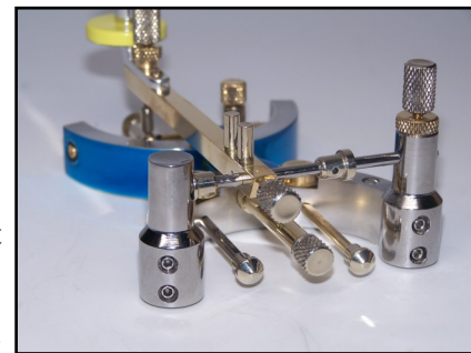
Photo #3: The rear of the key. The horizontal bar between the two posts is the torsion bar. The clamp which anchors the torsion bar sits atop the post on the right side of the photo. Three rods exit at the bottom: the center rod is one of the key's two binding posts for electrical connection. The smaller rods to left and right of this, are the two spare torsion bars in storage.
