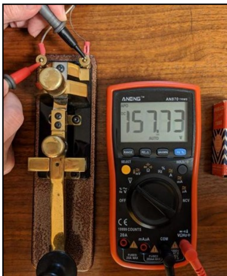
Voltage on the key before Keyall installed
