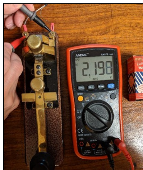
Voltage on the key after Keyall installed
