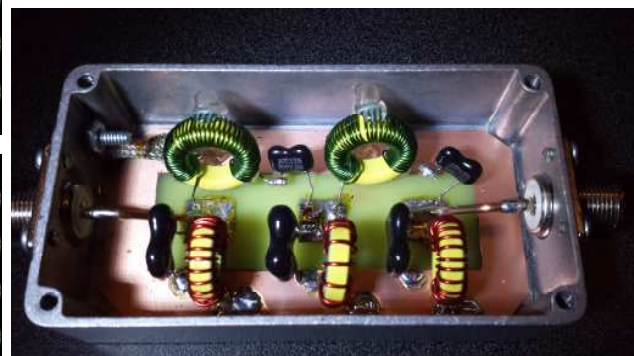
80m bandpass filter showing the smaller wire used to get the correct number of wraps on the toroid...made by KD8VSQ
