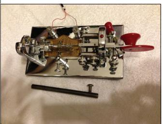
Here is the bug in position with the "speed control" installed.
