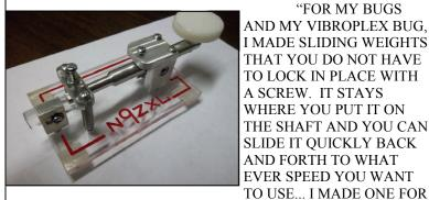
"FOR MY BUGS AND MY VIBROPLEX BUG, I MADE SLIDING WEIGHTS THAT YOU DO NOT HAVE TO LOCK IN PLACE WITH A SCREW. IT STAYS WHERE YOU PUT IT ON THE SHAFT AND YOU CAN SLIDE IT QUICKLY BACK AND FORTH TO WHAT EVER SPEED YOU WANT
