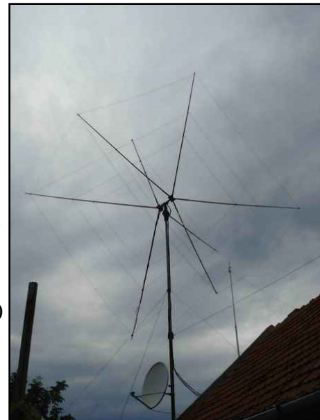
Two element triband quad at 32 ft
