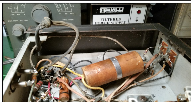
A frayed power cord and some aged capacitors were all that was needed to put an old receiver back on the air.
