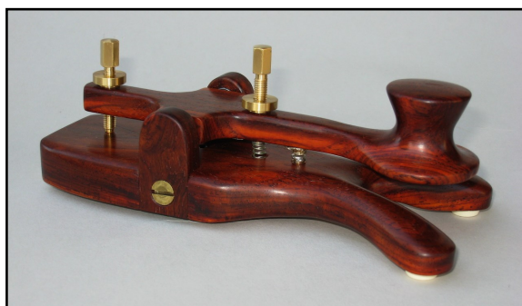
Figure 1. Morse hand key, made by the author in 2008. Cocbolo.
